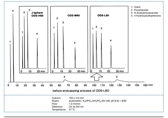
Three types of ODS are processed by endcapping technology to minimize the effect of residual silanol as much as possible.
