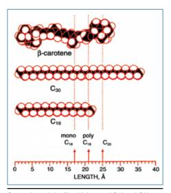
Comparison of the film thickness of C18 and C30 stationary phases with the molecular length of  $\beta$ -carotene (determined with Small Angle Neutron Scattering (SANS)).
